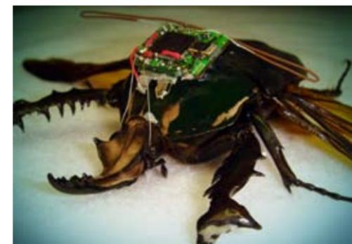
A beetle with neural stimulator implants and a radio-control board mounted on its thorax. *Hasta la vista, baby.*
