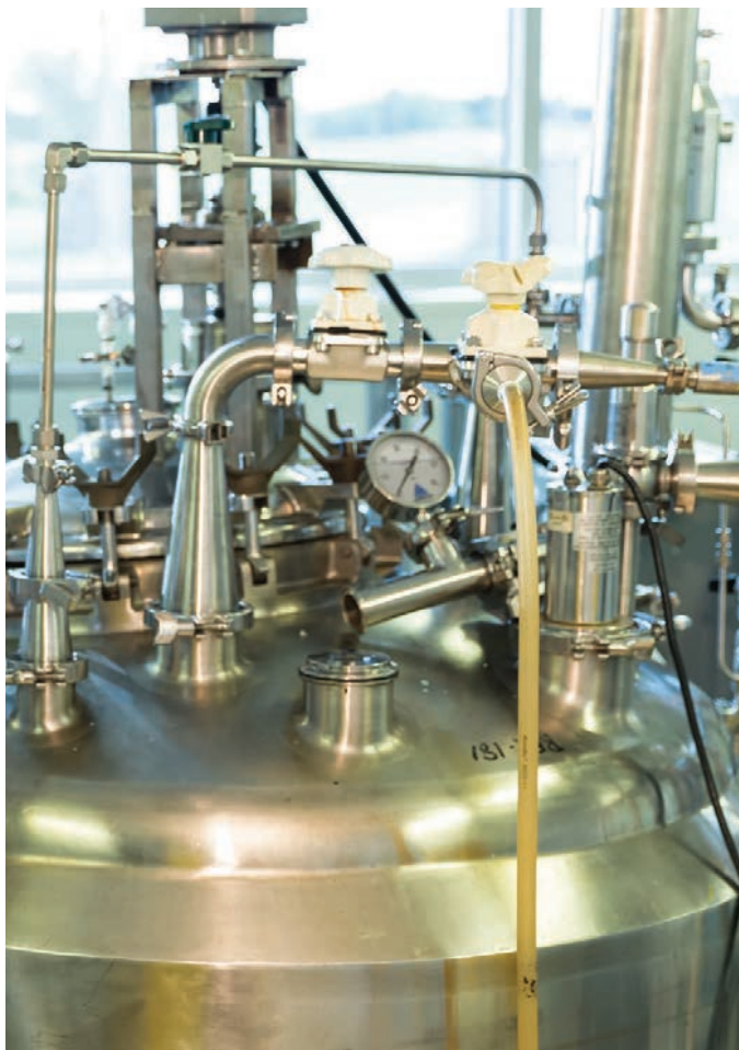
TerraVerdae's Edmonton production facility is equipped with a 2,000 litre pilot-scale bioreactor.
