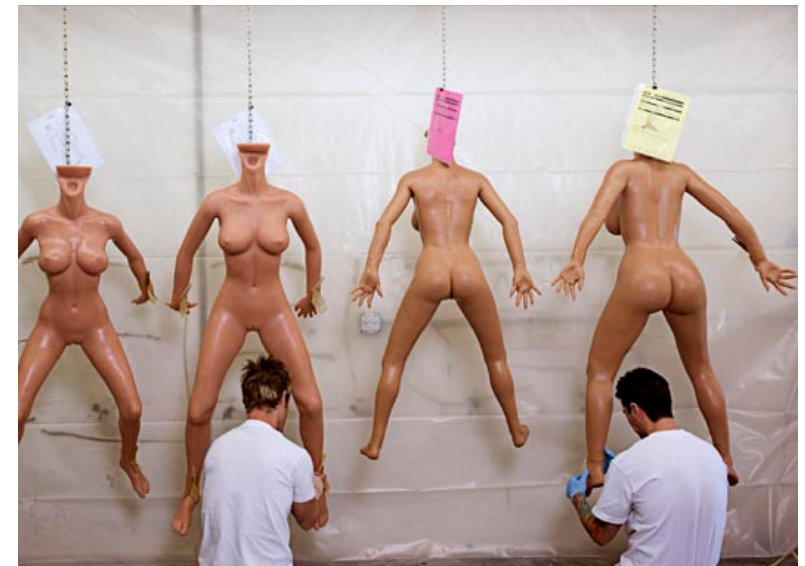
Two employees are patching the ankles where the dolls get bolted into the molds to prevent slipping, at Abyss Creations, a company located in the wealthy town of San Marcos in Southern California, which manufactures "the world's finest love dolls". These expensive life-sized silicone dolls (which cost USD $7,000 each), are made by hand.
