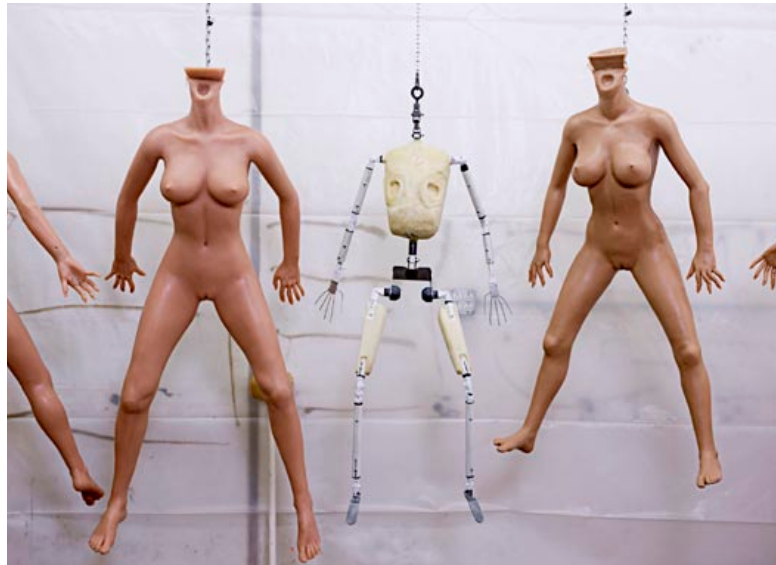
Abyss Creations, a company located in the wealthy town of San Marcos in Southern California, manufactures "the world's finest love dolls". The silicone is applied onto the underlying jointed framework.
