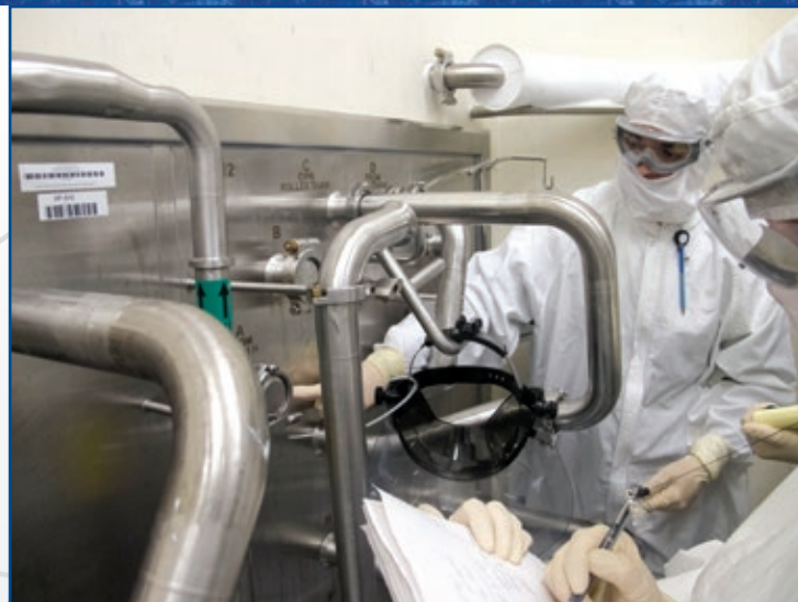
A biomanufacturing expert at Baxter's California plasma fractionation facility demonstrates to Quick Start's project study team how to operate the transfer panels used to control production processes.
