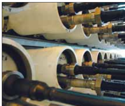
Membranes used for osmotic power are coiled inside tubular pressure vessels.
