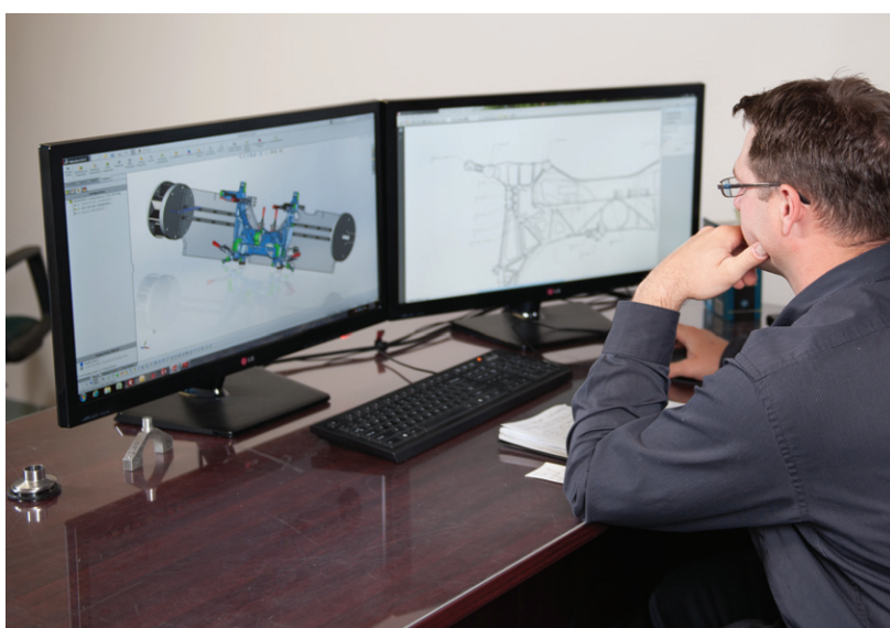
Chris Ferket, engineering manager, designs a fixture to hold an engine cradle for the Chevrolet Volt.
